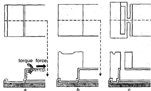
Fig. 2 Torque on suspended membrane owing to stress induced force, proposed firm anchoring structure using thick electroplating and advanced anchoring structure using thick electroplating to form springs having low series resistance
