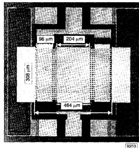
Fig. 3 Photograph of two-gap tunable MEM capacitor with firm anchoring
