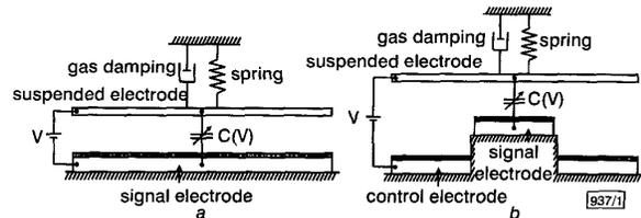
Fig. 1 Functional models of one-gap and two-gap MEM capacitors
