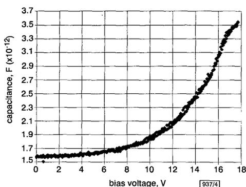
Fig. 4 Measured capacitance against voltage behaviour of two-gap MEM capacitor
