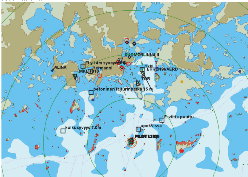
Figure 2. A screenshot from a maritime situational picture system. Vessels are visualised as triangles with the name tag on the upper-right corner. Squares are temporary obstacles.
