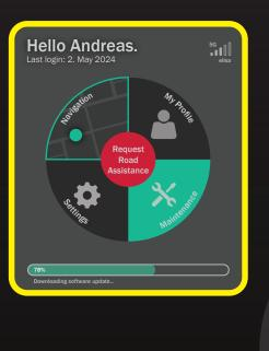
Immediately after a successful identification, the driver is presented with an interface that includes the most vital options and information: navigation, personal profile information, maintenance-related tasks, settings, and the ability to request an immediate dispatch of an official in the case of an emergency or technical failure. The next pages will elaborate on the features of the interface more thoroughly.
