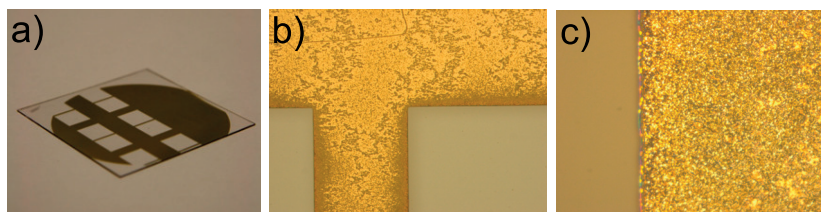
Figure 6.8. a) Image of the patterned Ag nanoparticle sample, b) 5x and c) 50x magnification optical microscope image of patterned Ag nanoparticle structures.
