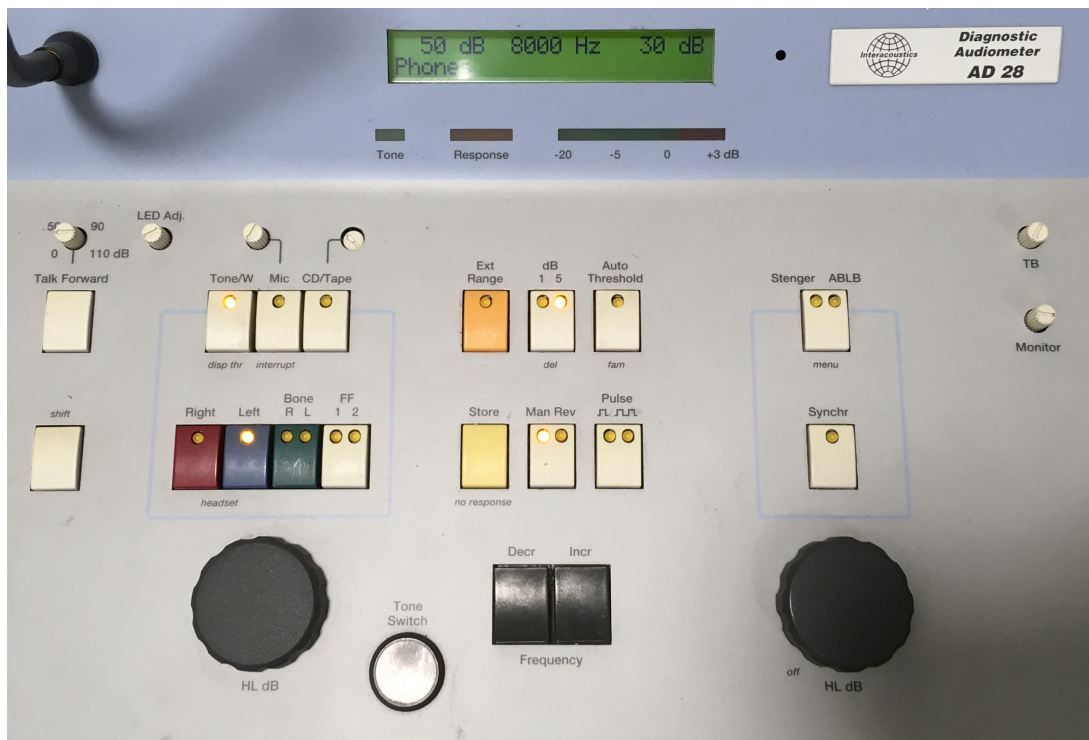
Figure 12: Close-up of the front panel of the Interacoustics Diagnostic Audiometer Model AD 28.
