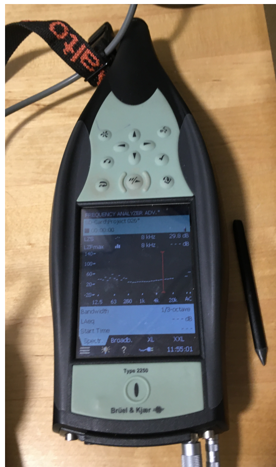
Figure 14: Brüel & Kjær Hand Held Analyzer 2250. It was used as the sound pressure level meter when calibrating the audiometer.
