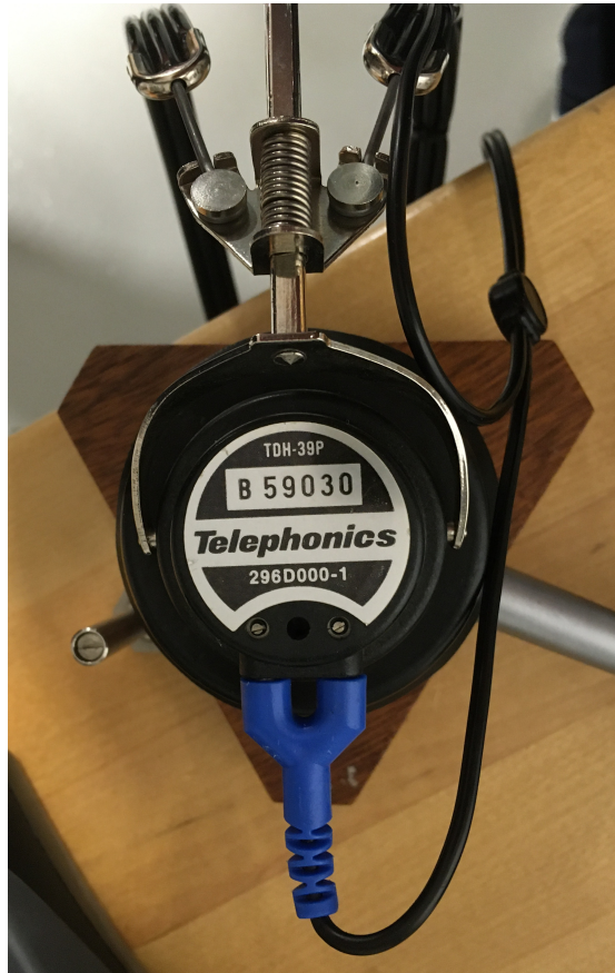
Figure 16: Telephonics TDH-39P Audiometric Earphones, positioned on top of the Brüel & Kjær Artificial Ear 4153 shown in Figure 15.
