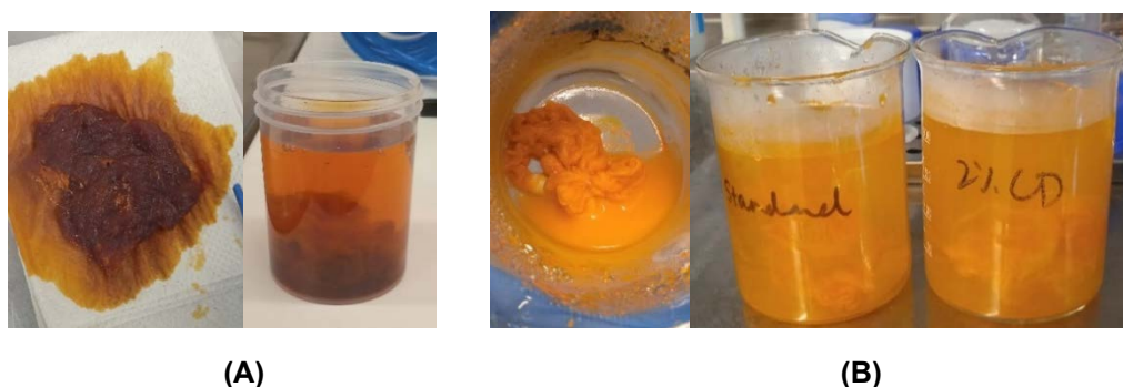
Figure 5: Dyeing of spun fibres with curcumin. (A) Dyeing with 2%(v/v) NaOH and 1% curcumin solution. The first image shows the fibres after dyeing before washing. The second image is the washing water containing released dye; (B) Dyeing with 30%(v/v) ethanol and 1% curcumin. The first image is after the dyeing procedure and before washing. The second and third image shows the release of the dye to the washing water.
