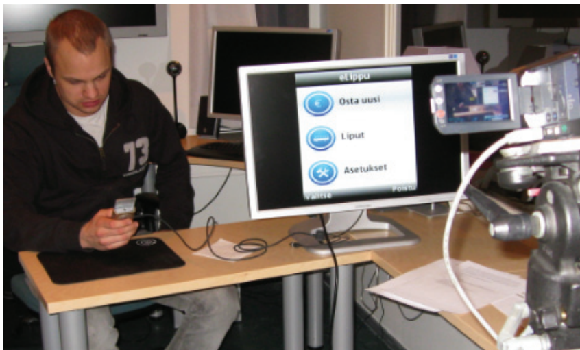
Figure 18: A separate monitor was used so that the moderator could see the user's actions with the phone, and get a good video recording even if the user moved the phone.
