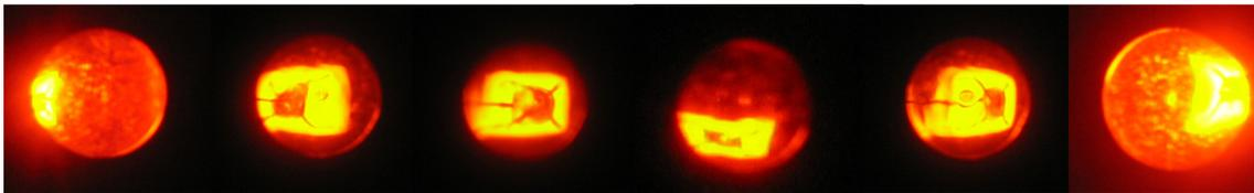
**Figure 17.** Photograph of the virtual source of an orange 10-mm LED taken in different directions. The third photograph from the left shows the image source on the optical axis.
