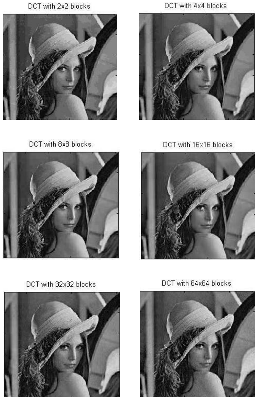
Figure 18: Lena with different blocks size of DCT
