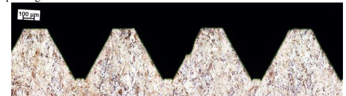
Figure 21: AB plate, M5, pre-hole diameter 4.3 mm, up-skin thread, objective 10 X, 90° printing inclination
