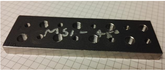
Figure 19: M5 and M8 threads in ST maraging steel plate
