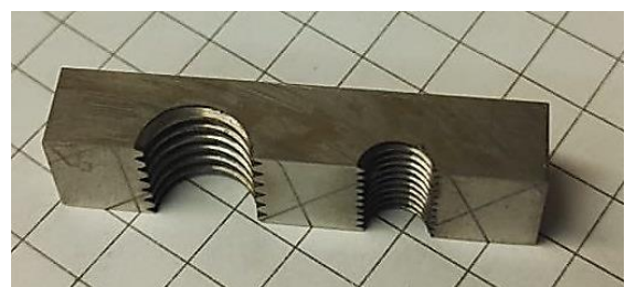
Figure 3: The sectioned internal threads for optical microscopic imaging
