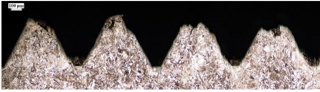
Figure 25: ST plate, M5, pre-hole diameter 4.3 mm, down-skin thread, objective 10 X, 90° printing inclination
