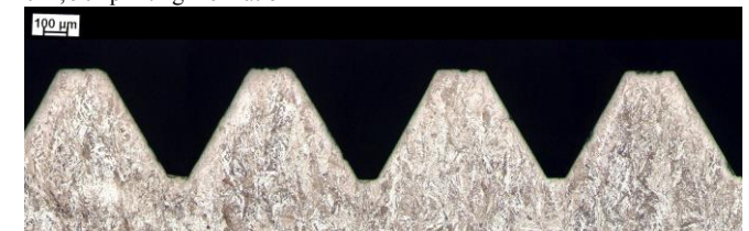
Figure 22: AB plate, M5, pre-hole diameter 4.3 mm, down-skin thread, objective 10 X, 90° printing inclination
