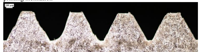
Figure 24: ST plate, M5, pre-hole diameter 4.3 mm, up-skin thread, objective 10 X, 90° printing inclination
