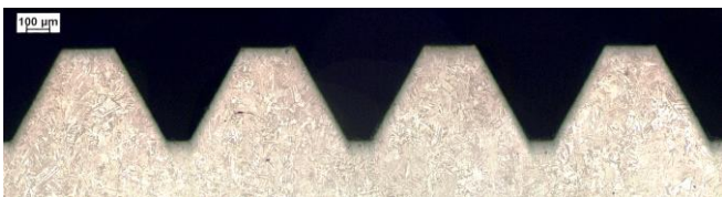
Figure 29: AB+Aged, M5, pre-hole diameter 4.3 mm, down-skin thread, objective 10 X, 90° printing inclination
