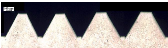
Figure 28: AB+Aged, M5, pre-hole diameter 4.3 mm, up-skin thread, objective 10 X, 90° printing inclination
