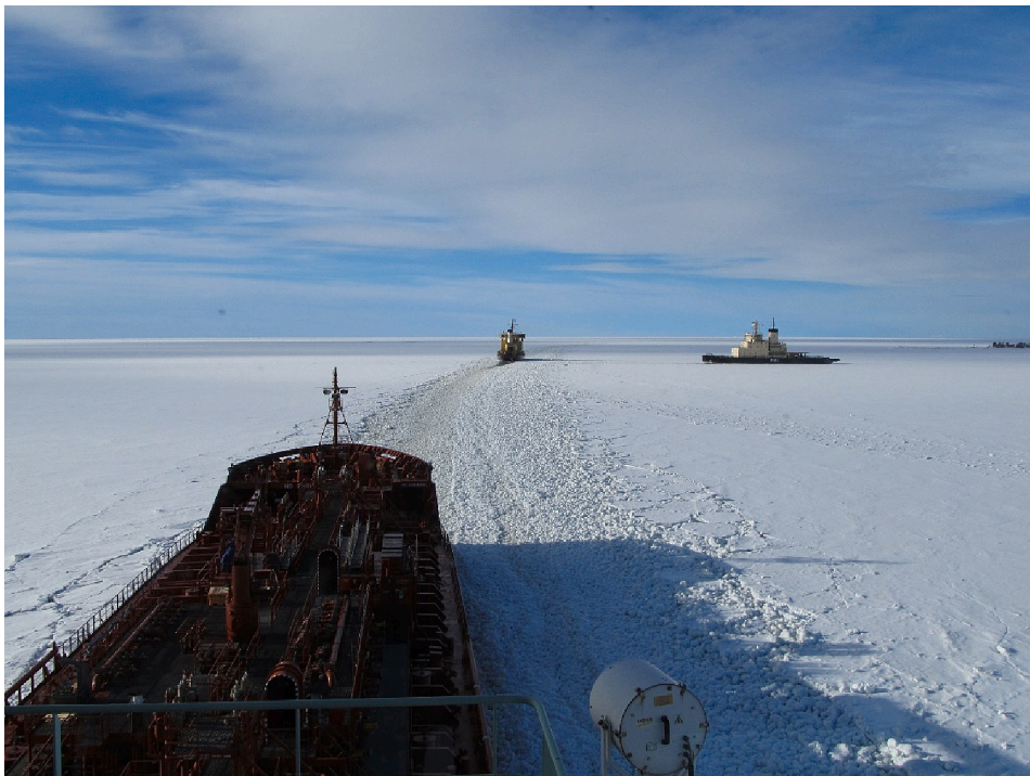
Fig. 1. An icebreaker assisting a merchant ship in an old brash ice channel at the Baltic Sea.
