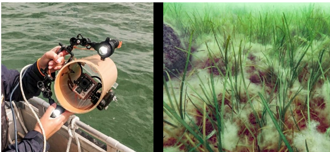
Figure 16: Submersible part of an action camera-based self-made dropvideo system developed by Husö biological station with an image of the bottom [43]
