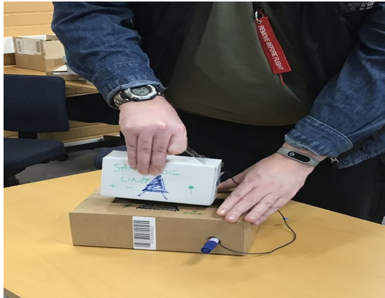
Figure 23: The sampling unit (white) can be removed from the housing (brown)
