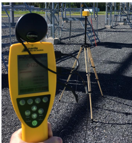
Figure 2: The Narda NBM-550 broadband field meter in the front, and the Narda EHP-50F electric and magnetic ELF field probe in the back.
