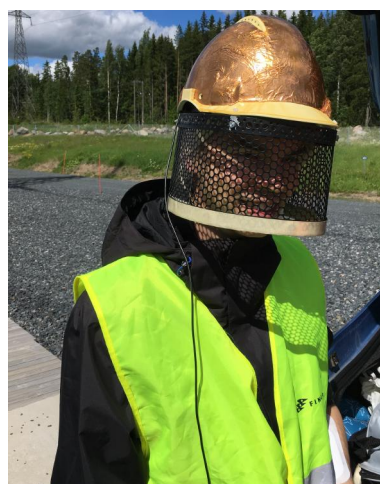
Figure 3: The helmet-mask measurement system being worn.
