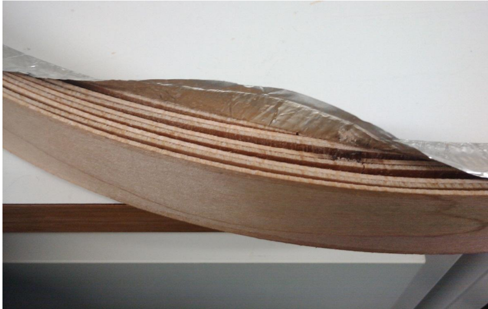
Figure 40 Delamination of the specimen 18 M 3 after oven-drying
