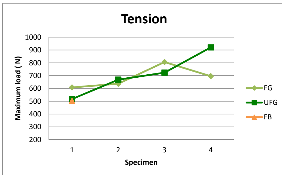
Figure 58 Tension test for formed specimens
