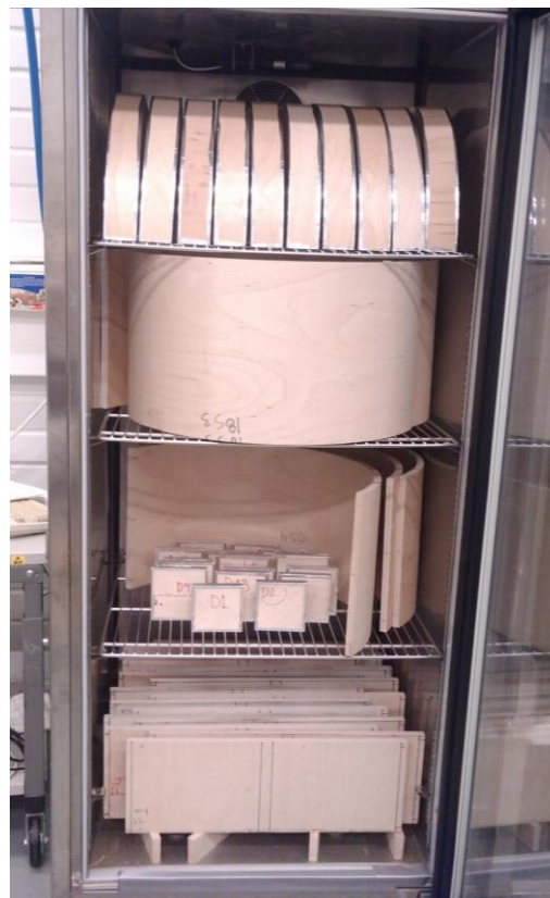
Figure 17 Conditioning cabin one, specimens inside; from the first grill: edge sealed formed specimens, diameter change specimens, edge sealed formable and UF specimens, and in the bottom the flatness specimens
