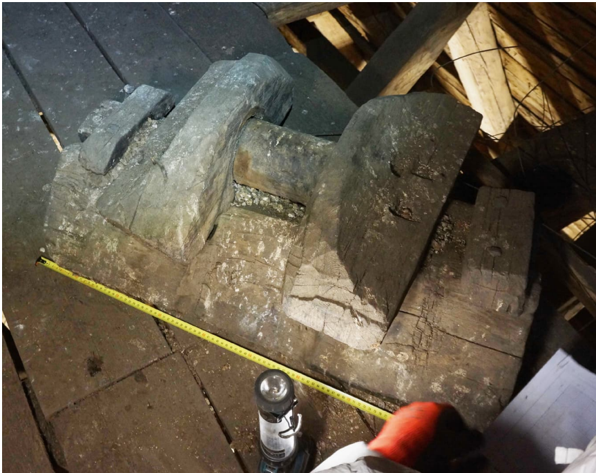
FIGURE 16 The winch found in the attic of Karjaa Church PHOTO BY MIINA TOLONEN (2020)
