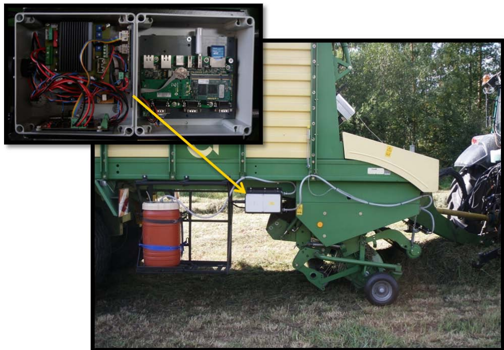
Figure 21: The additive applicator with an additive container mounted on the side of the loader wagon. The nozzles are installed on the cut-and-feed unit.
