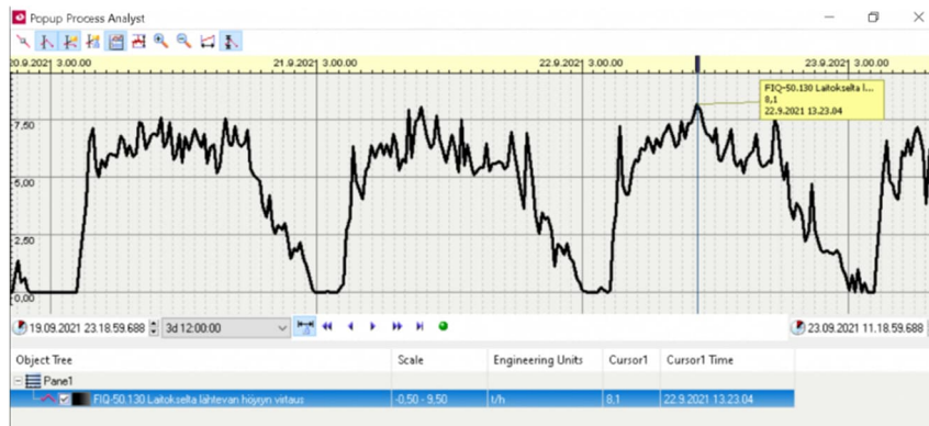
Figure 29: Hourly steam consumption from Tuesday 21.9.2021 to Wednesday 23.9.2021
