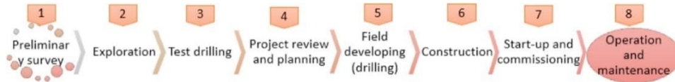
Figure 2: Eight stages of geothermal heat project according to ESMAP and WBG (Moya et al. 2018)
