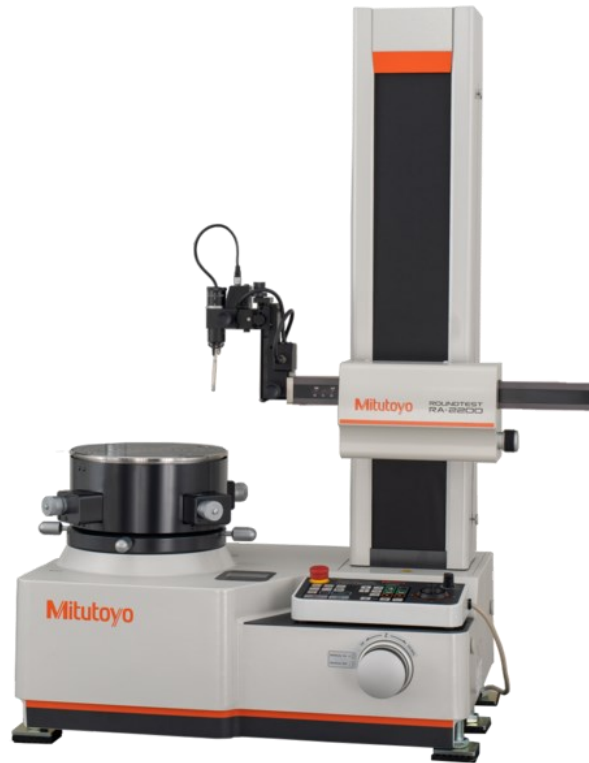
Figure 2.3: A cylindricity measuring instrument (Roundtest RA-2200AH, 2024).
