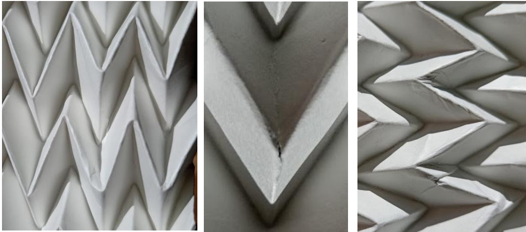
Figure 63. Few defects of the previous samples a) Unsharp folds at the edge of the sample b) Small rupture in the corner point c) Unsharp folds and uneven mountain lengths
