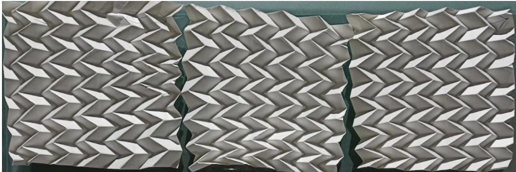
Figure 60. Three 20 cm x 20 cm samples made from 170 g/m 2 paperboard in transverse pattern orientation
