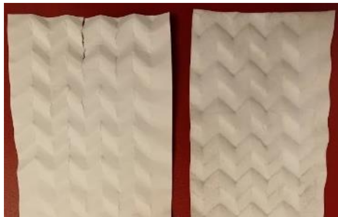
Figure 52. Test of dry and wet paperboard samples ran through roller nip prototype 5
