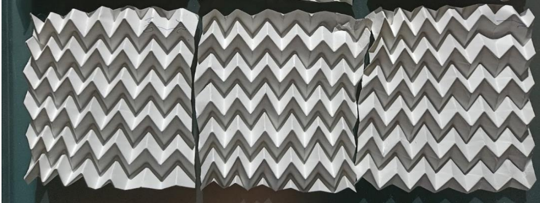
Figure 61. Three 20 cm x 20 cm samples made from 170 g/m 2 paperboard in longitudinal pattern orientation
