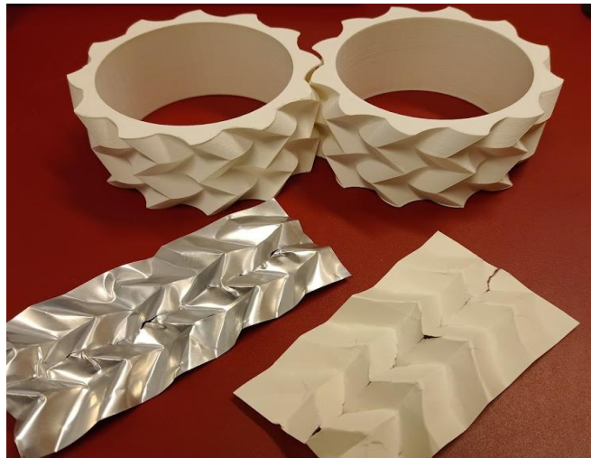
Figure 37. Second iteration of TPO roller nip and the samples of aluminium and paperboard
