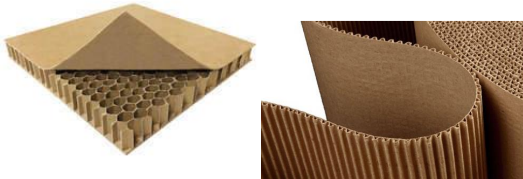
Figure 2. a) Honeycomb structure (rebul.com, 2023) b) Corrugated cardboard (lakkapaa.com, 2023)
