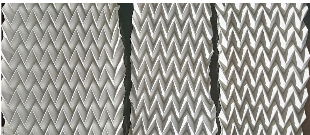
Figure 64. 20 cm x 50 cm samples made from 170 g/m 2 paperboard. The two samples on the left were made using re-re-wetted paperboard and the sample on the right was made using dry paperboard.
