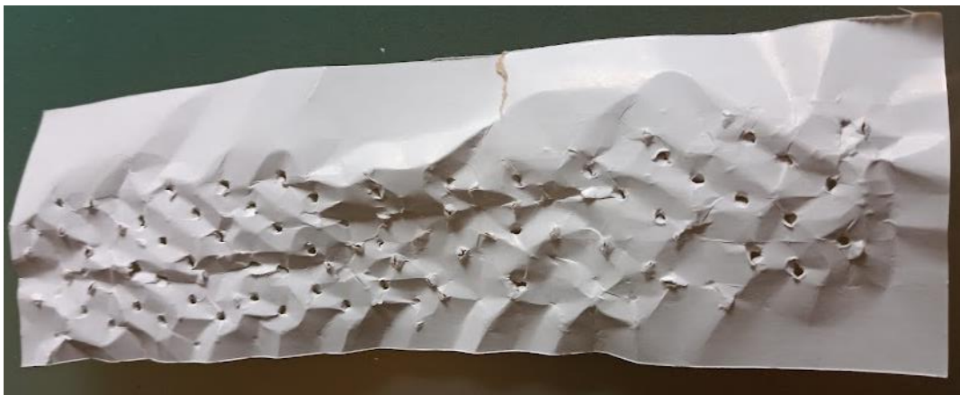
Figure 40. Punctured paperboard sample from spike rollers
