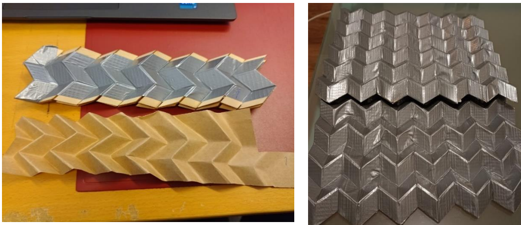
Figure 48. a) 0.8 mm plywood parallelograms attached to duct tape b) Two Miura-ori mats made from plywood and duct tape
