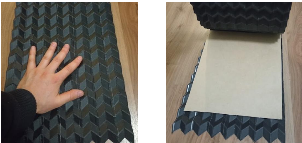
Figure 54. The foldable mats are spread as flat as possible. Then the material is placed between the mats.
