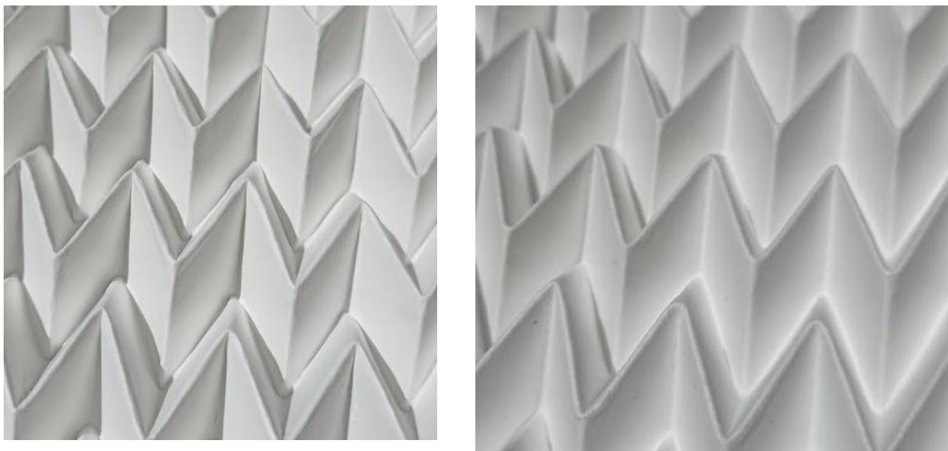
Figure 65. Close up photos of folded a) dry paperboard b) re-wetted paperboard
