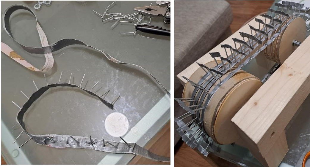
Figure 43. a) Manufacturing of the spiked belts folding machine
