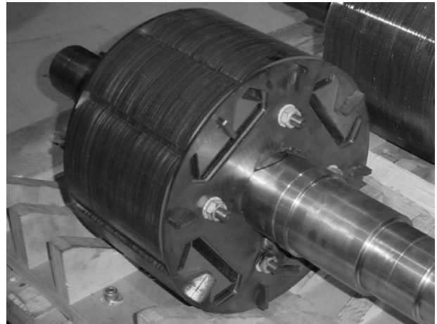
Fig. 12. Prototype of eight-pole rotor with bridges.
