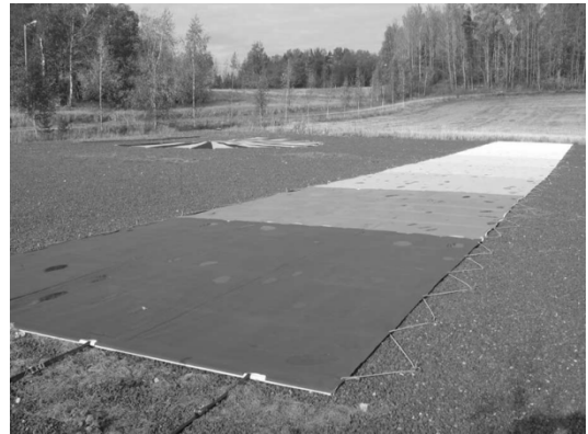
Fig. 2. Targets arranged in a line at the Sjököla photogrammetric test field in Kirkkonummi (see [15] for more details) while testing a digital aerial camera. (Photo by H. Kaartinen, FGI.)
