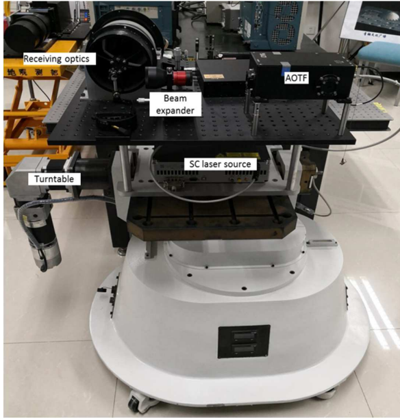
Figure 4.10. AOTF-HSL system for the field test on a two-dimensional turntable.
