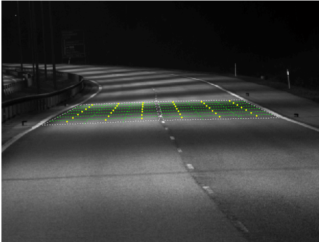
Fig. 7. Pilot location on VT1 illuminated with MH lamps. Luminances of the pilot location are shown in gray scale map. The Custom 2 method is used for the calculation of average road surface luminance, overall luminance uniformity and longitudinal luminance uniformity. Each lane is divided to 21 measurement points; 3 points in the transverse direction and 7 points in the longitudinal direction. For each point the luminance value is calculated by using the average luminance value of all pixels that are located in the rectangle of the relevant point (“Equal area”).
