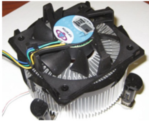
Figure 21: Typical axial fan used in LED cooling [18]
