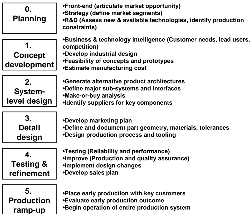
Figure 18: Ulrich and Eppinger’s (2000) different phases and main activities of a product development process
