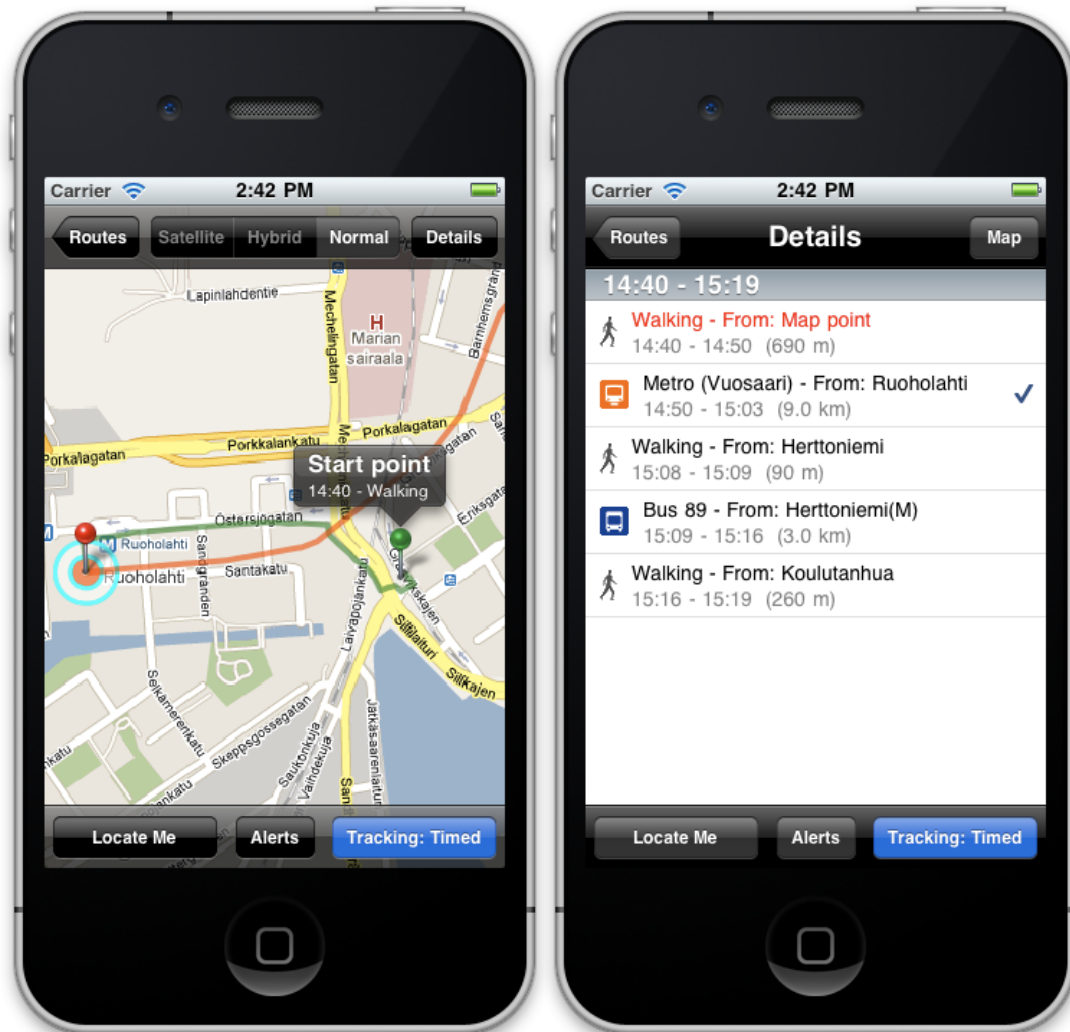
Figure 9: Left: The paths of different legs of the route crossing. Right: A list of the legs of the route. Check mark indicates the currently selected leg. Tracking status is ‘Timed’ instead of ‘ON’ because the departure time for the chosen leg has not yet passed.
