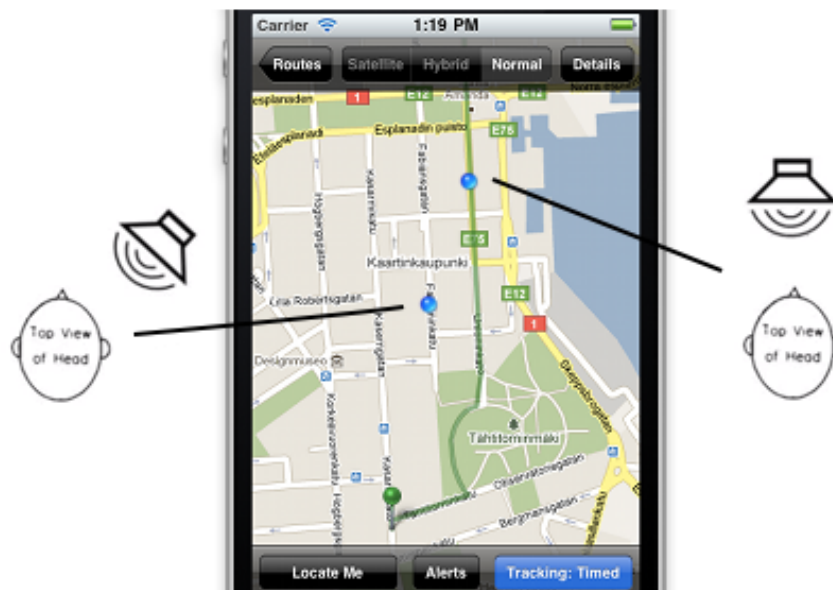
Figure 11: Direction of the sound of footsteps panned towards the path.
