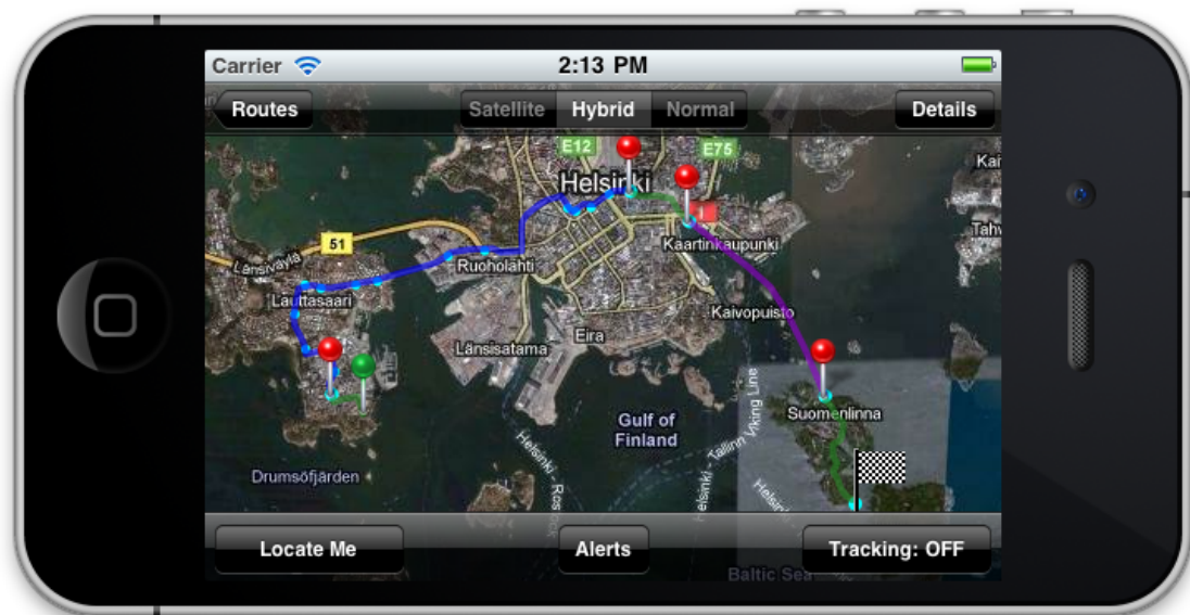
Figure 5: Different parts of the route are drawn with a color representing the type of transportation.
