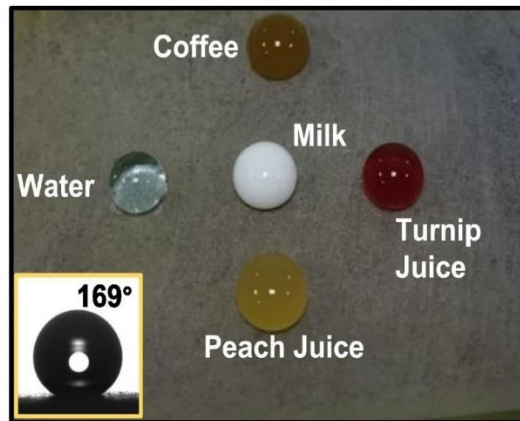
Figure 6: Contact angle characterization of the fabricated surface. Droplets of selected liquids bead up to indicate superhydrophobicity, and the water contact angle indicated as 169^\circ [16].
