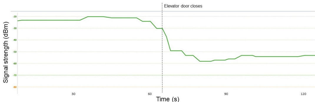
Figure 15. Wi-Fi signal strength inside the elevator car with the AP close to the elevator shaft. Signal strength is better than in Figure 14, but still it diminishes significantly when the elevator car doors are closed.
