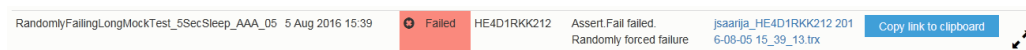
Figure 5.2: As a workaround for accessing test results logs on Test Executions page, a separate button for copying link to the test log into user's clipboard was provided on the right side of each test execution item.
