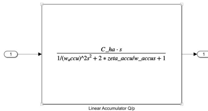
Figure 9. The accumulator subsystem consists of a transfer function presented in equations 27 and 28.
