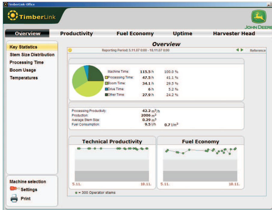
Figure 7.5: An example of the TimberLink user interface. In the bottom of the screen time series index data for technical productivity and fuel economy is shown.
