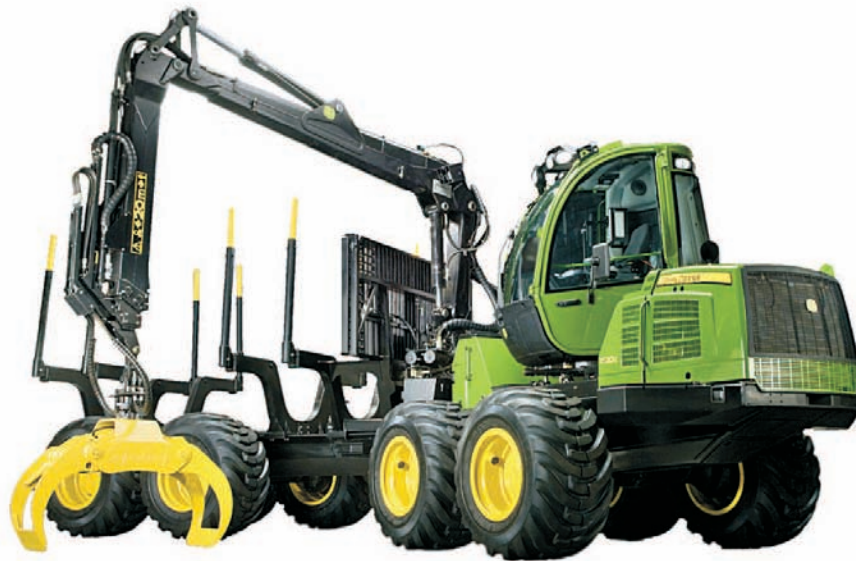
Figure 7.2: A forwarder which is used for carrying the logs to the roadside.
