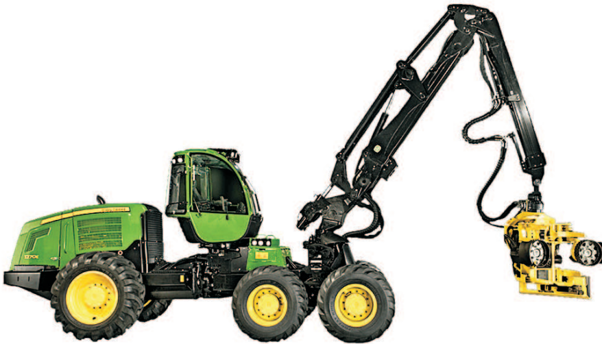
Figure 7.1: A cut-to-length forest harvester which is used for felling and delimiting trees and cutting them into logs of predetermined length.
