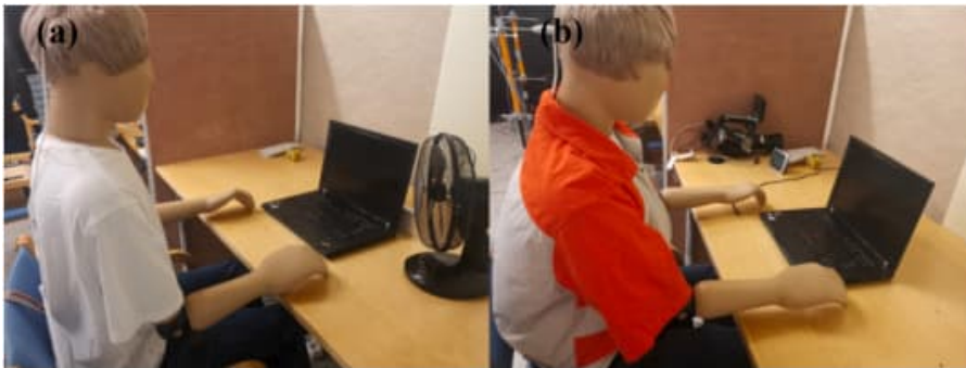
Figure 5. Thermal manikin test with (a) the table fan and (b) the air-cooled jacket. (the evaporative cooling device positioned identically to the table fan.)
