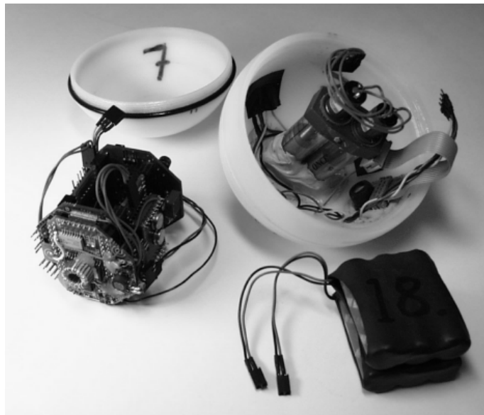
Figure 4.4 SUBMAR electronics unit, casing, and battery packs.
