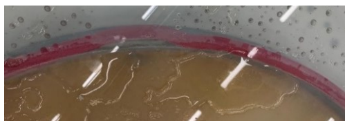
Figure 4.9 Displaced rubber ring due to high water pressure.
