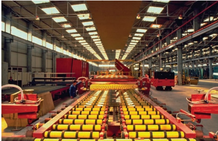
Figure 2.3 Thickness control of glass ribbon through rotating rollers [15].
