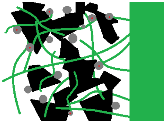
Figure 13. Schematics of the CL structure and the 3-phase boundary with solid electrolyte. Green: the membrane and the ionomer, black: carbon, grey: catalyst particle. Particles marked with red are active due to simultaneous access to carbon, ionomer and pores.
