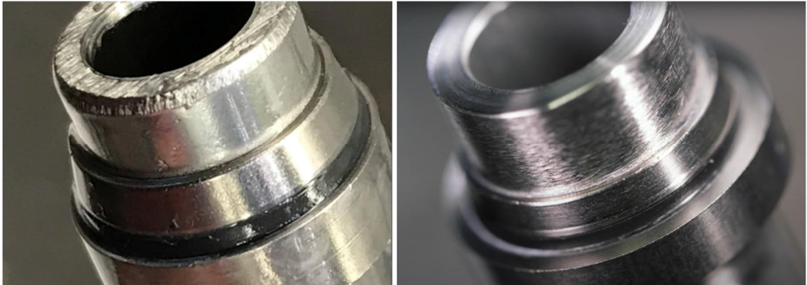
Figure 28. Case company pre-assembled cutting ring versus correctly pre-assembled ring.
