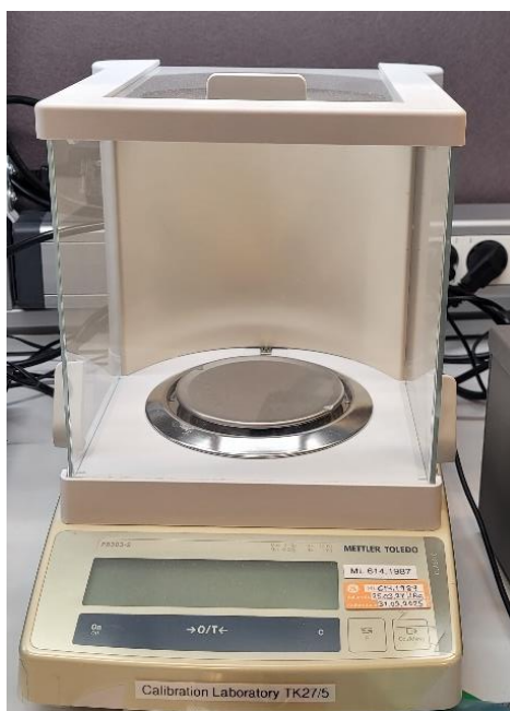
Figure 23: Scale used in battery weight measurements
