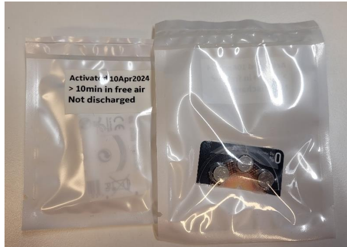
Figure B1: Heat sealed CPP/OPP laminated bags
