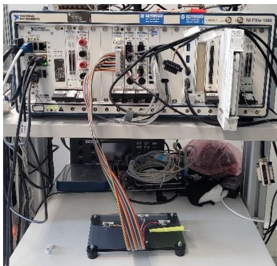
Figure 22: The complete setup for discharge tests with fluctuating current
