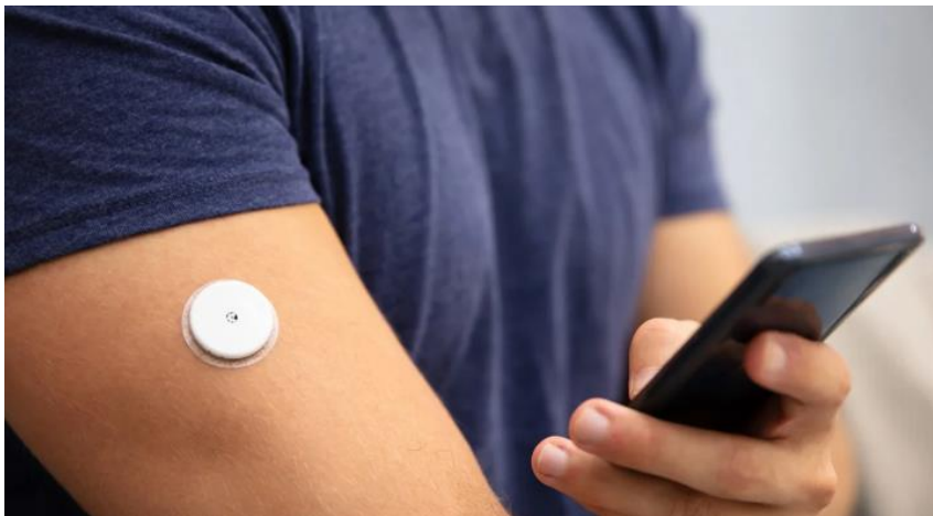
Figure 1: The Abbott FreeStyle Libre continuous glucose monitoring sensor [11]
