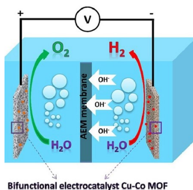
Figure 16. Schematic diagram of bifunctional electrocatalysis of Cu-Co MOF [54]
