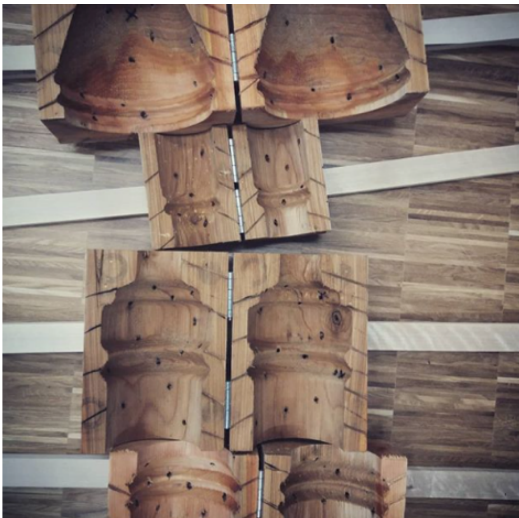
Figure 4. Wooden moulds were cut from a fresh alder that Espoo city kindly gave me. Photo by author, 2018.
