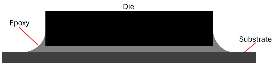
Figure 1: Illustration of epoxy die bonding.
