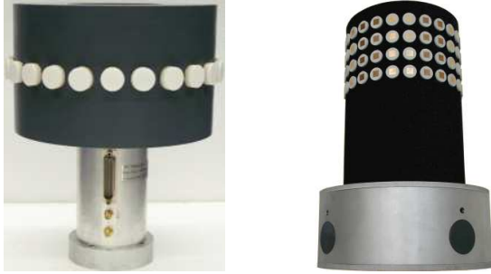
Figure 4: On the LHS, Polarimetric Uniform Circular Patch Array (PUCPA) with N = 24 patch elements. On the RHS, Stack Polarimetric Uniform Circular Patch Array (SPUCPA) with N = 24 patch sensors. Courtesy of TU-Ilmenau.
