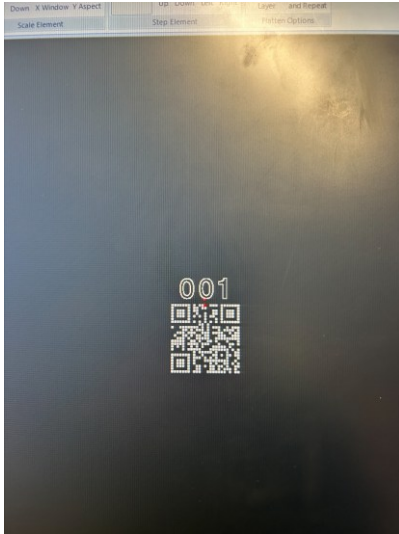
Figure 16: Laser Engraving Direct Part Marking
