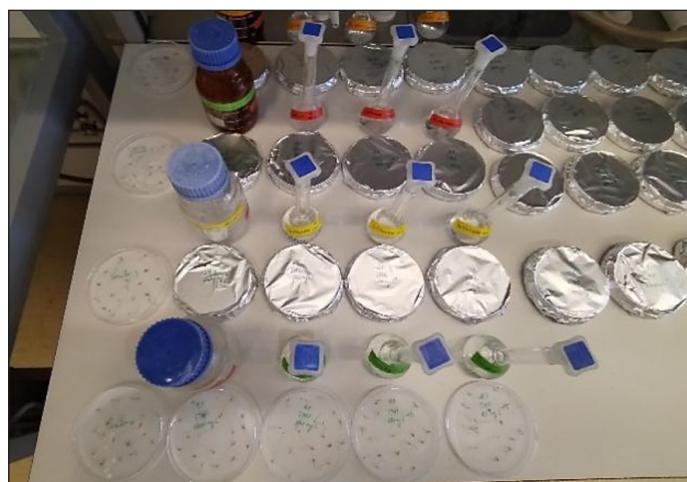
Figure 1. Preparation of sample drug solutions from each of the 4 concentrations to determine acute toxicity, experiments were carried out with four concentrations of the drug, i.e. 0.1, 100, 500 and 1000 mg L -1 , which were obtained from serial dilutions in triplicate, and distilled water was used for control growth in a total amount of 78 experimental units (Fig. 2).
