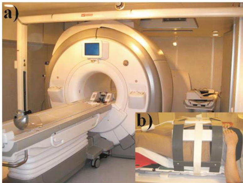
Figure 1. The MR simulator in HUCH Cancer Center (2011). a) shows the scanner with the goal-post laser system, and b) presents patient positioning for pelvic imaging with MR-compatible immobilization. The anterior part of receiver coil is attached to the constructed frame, and posterior part of the coil is placed below the flat table top.
