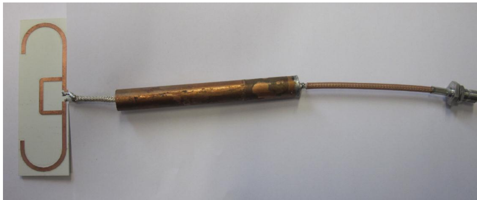
Figure 33: Photograph of the Zero Power sensor antenna.
