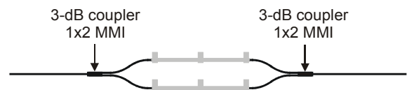
Fig. 2 Mach-Zehnder Interferometer with two 3-dB 1x2 MMIs. The grey areas represent the heaters.
