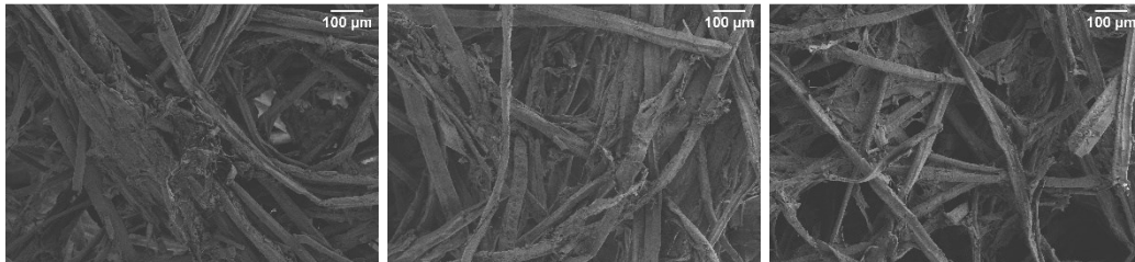
Figure 34. Sample C1 (two first ones) and C2 (the last one) with magnification of 100x showing denser surface of the samples.
