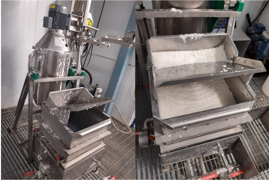
Figure 15. A foaming tank used to prepare the fibre foam (left). Foam poured along a tilted plate into a rectangular sheet mold (right).
