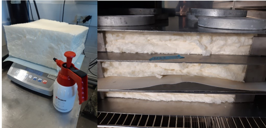
Figure 16. Dry sample was re-wetted into 50% dry matter content (left). After re-wetting, the samples were pressed into desired thickness with a dynamic press and were dried overnight in the oven (right).
