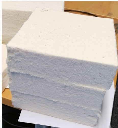
Figure 17. The samples were cut into four pieces of size 18 cm x 18 cm and left in standard test conditions ( 23^{\circ}\text{C} RH 50%) for 4 hours before drop tests.
