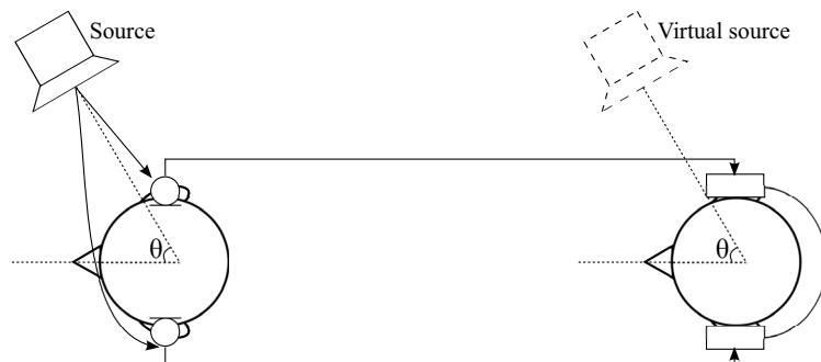
Figure 3.7. Principles for the binaural recording.
