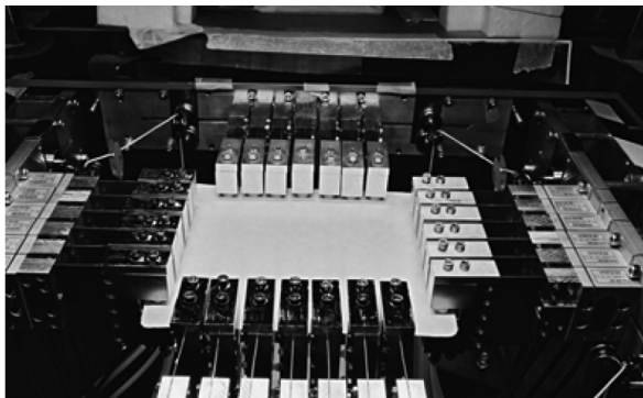
Fig 1. The Paper Drying Rheometer (PDR) with an attached test sheet.
