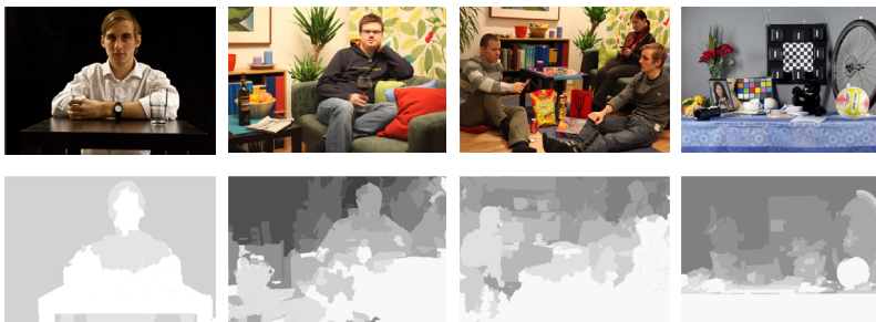
Figure 4.14. Scenes in the following order: “Bar”, “Wine”, “Game” and “Composition.” The first row shows the S3D scenes used in this study. The bottom row shows the depth maps. The white values correspond to the nearest depth and the darkest values to the farthest depth. The depth maps were computed separately for each scene and should not be compared.
